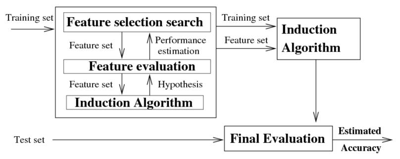
The induction algorithm itself is used as a "black box" by the subset selection algorithm.
