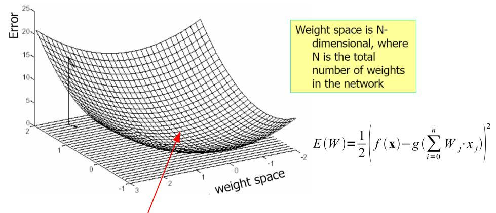
The best weight setting for an example is where the error measure for this example is minimal
