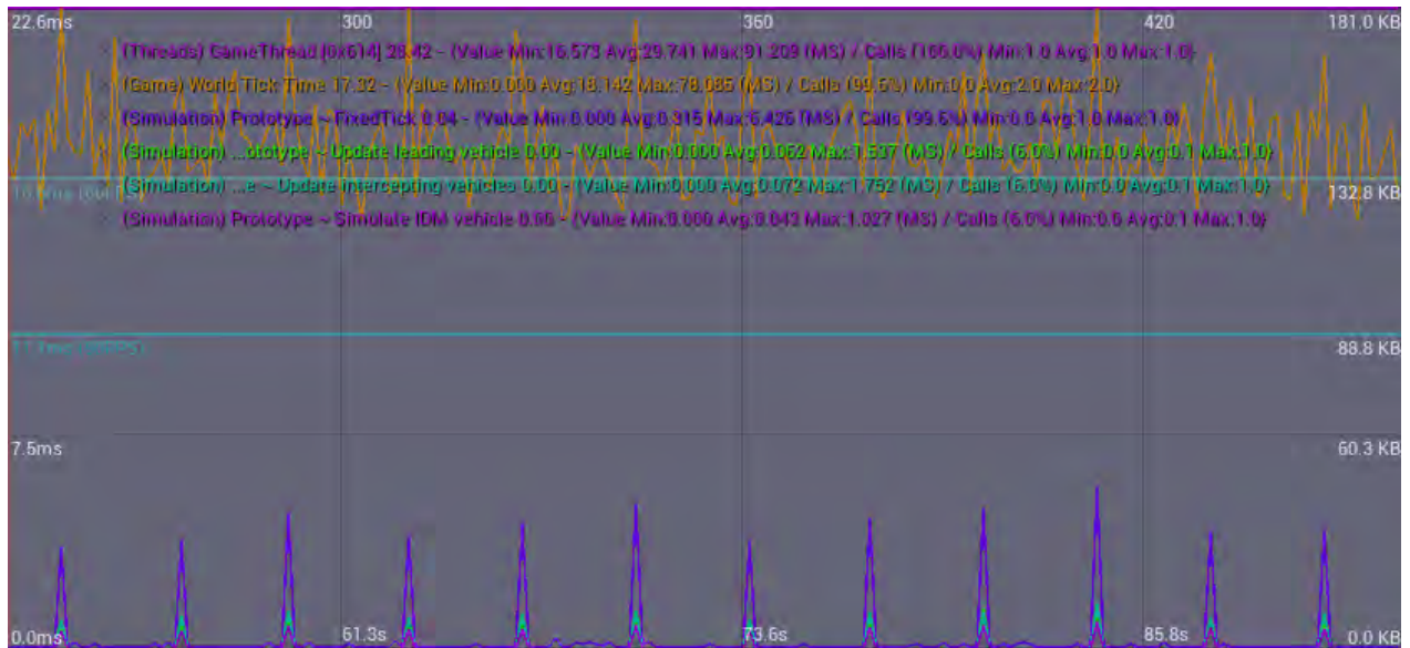
Figure 6.8.: Profiler graphs of a curvy scenario with about 2000 vehicles on 32 km of road simulated with improved sorting show frame times of (from top to bottom): All game logic added up (orange), simulation (violet spikes), which includes finding intercepting vehicles (cyan spikes), finding leading vehicle (green spikes) and acceleration calculation (purple spikes). The simulation performs better than it does with the old method of sorting but with an average of 18.142 ms per frame all game logic added up performs worse.
