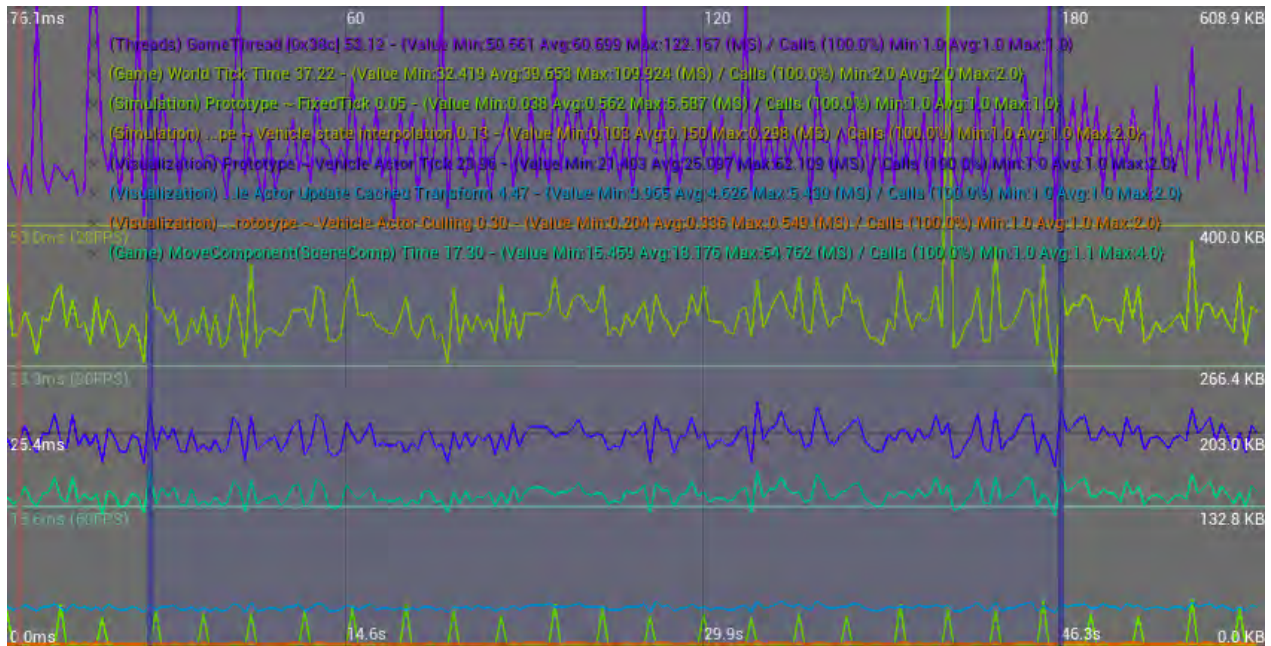
Figure 6.17.: Profiler graphs of 16 km of curvy road with about 2000 vehicles show frame times of (from top to bottom): All game logic added up (green), vehicle actors (purple), which includes moving actors (cyan) and calculating 3D location (light blue), simulation (green), interpolating simulated location (yellow). With MoveComponent taking an average of 18.176 ms each frame and the FixedTick taking a maximum of 5.587 ms every 0.5 s, hiding out-of-frame or far-away vehicles is far more efficient for this scenario than optimizing the simulation.
