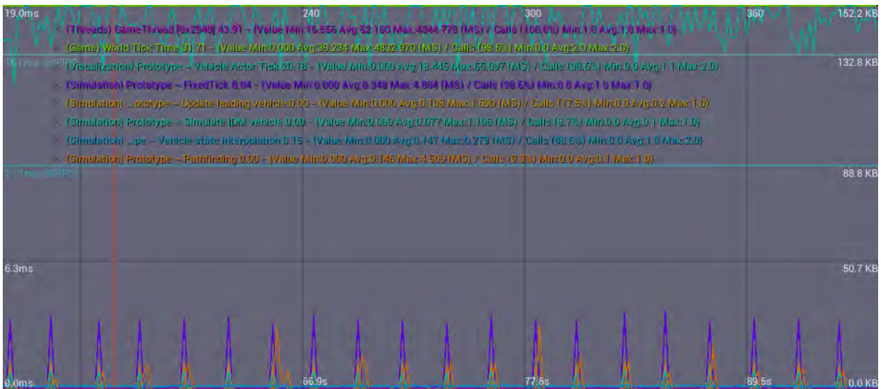
Figure 6.10.: Profiler graphs of a ten by ten city grid with about 2000 vehicles on 100 m road sections with disabled recognition of intercepting vehicles show frame times of (from top to bottom): All game logic added up (green), vehicle actors (cyan), simulation (violet), which includes finding leading vehicle (light orange) and calculating acceleration (cyan), path finding (orange), interpolating simulated location (blue). Although simulation takes much less time than it does with enabled lane-changing model, all game logic added up is not performing well enough with an average of 39.234 ms per frame.
