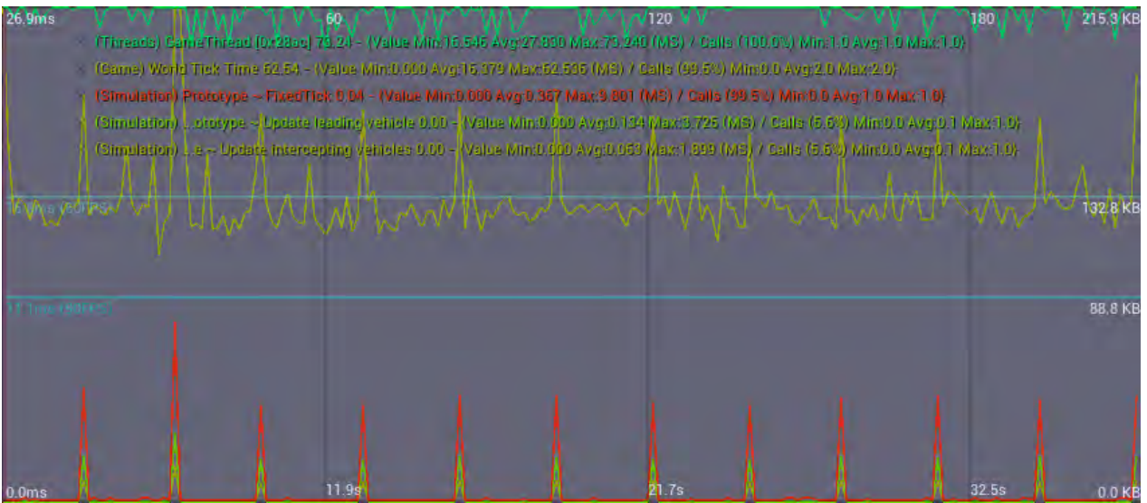
Figure 6.6.: Profiler graphs of a curvy scenario with about 2000 vehicles on 32 km of road with 500 m sections show frame times of (from top to bottom): All game logic added up (yellow), simulation (orange spikes), which includes finding leading vehicle (green) and finding intercepting vehicles (yellow). With all game logic taking an average of 16.379 ms per frame the game performs very smoothly.
