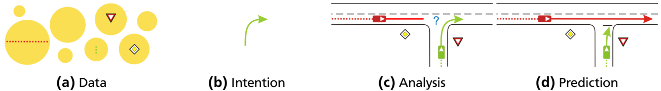
Figure 2: An example diagram for a possible outcome (d) in a traffic situations, where a system analyses (c) the traffic situation with the given data (a) and driver intention (b).
