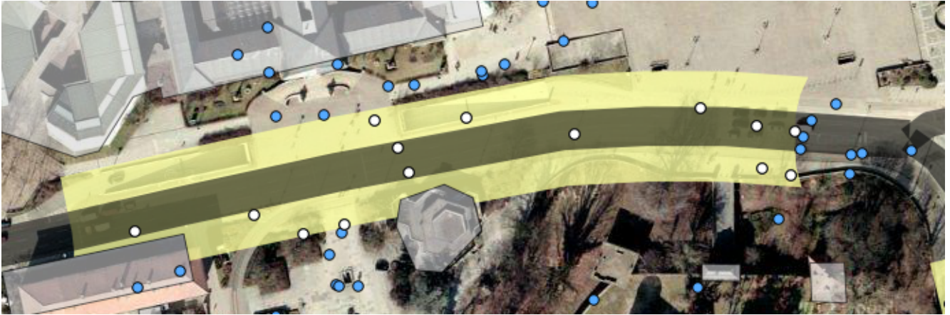
Figure 3: In the plan view above, the road segment geometry is displayed in black, the selection area in yellow and the geometry of the buildings in white. In this specific case, the selection area covers a space with a distance of 10 meters around the road and excludes the area in the proximity of 30 meters to neighboring road segments, as well as the area of the surrounding buildings. The recording positions of the non-selected measurements are displayed in blue, and those of the selected measurements in white. In this example, only measurements within the selection area are included for building the training examples.
