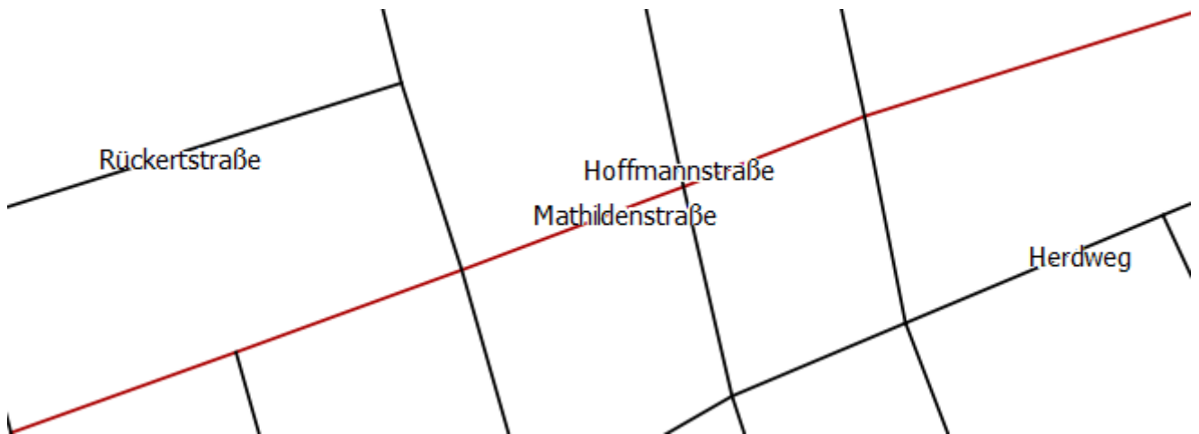
Figure 8: The raw OSM data describe non-planar network topology. E.g. A way describing Mathildenstraße, Darmstadt crossing other ways.
