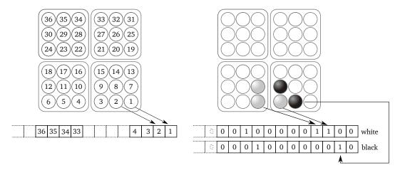
Figure 6.3: Linear mapping of each position in the board onto the bit string.
