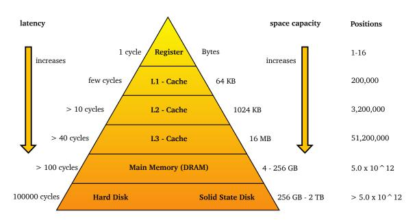
**Figure 5.5: Storage hierarchy** of actual consumer hardware. Unpredictable accesses to the main memory and especially to the Hard Disk are very time intensive. Thus, these so called cache misses should be avoided. The right most column expresses a rough estimation of positions which fit into the given space without Huffman encoding.
